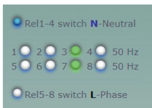
In the Power and Power 19" version, different supply systems can be connected for both sides (relays 1-4 and 5-8): e.g. 1-4 120VAC 60 Hz and 5-8 230VAC 50 Hz.
