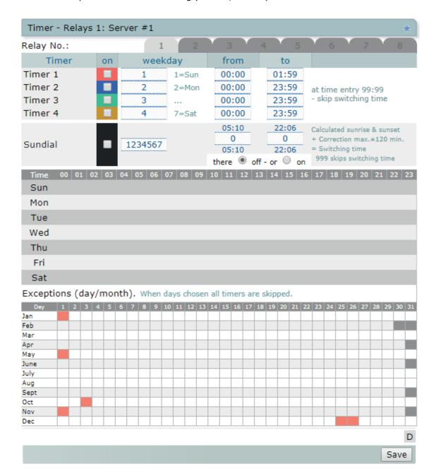
Sundial: The ,from' -'to' times are calculated automatically (2:00 AM) according to the information in the Time section. With: "In time off or on", it can be determined whether the relay should be switched: Is selected "In time off" = switched on at night - switched off during the day. If "On time" is selected = switched off at night - switched on during the day.
