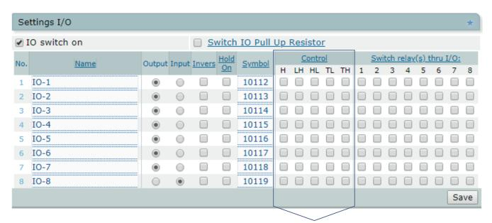
If the function: "Switch relay(s) thru I/O" is used, the "Control" function can be used to determine the type of control (edge) of the IO input when switching the relays:
